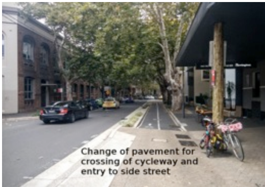
Bourke Street, Surry Hills: Separated cycleway along a neighbourhood street
